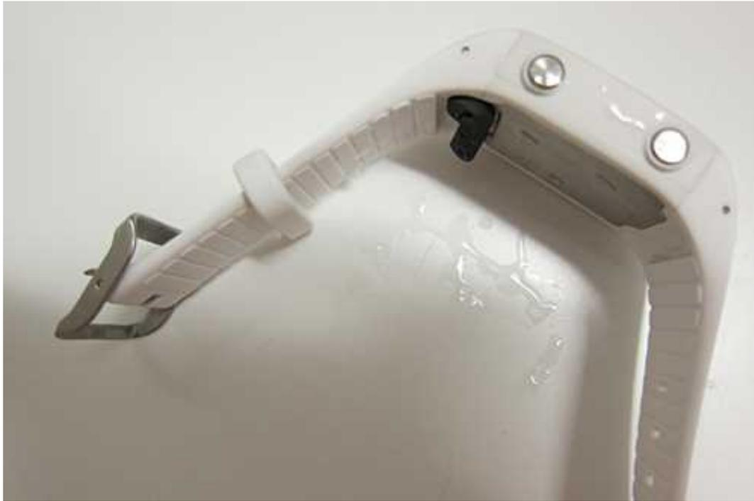
When using the USB port, check that there is no moisture, hair, dust or dirt on the sealing surface area. Gently wipe off any dirt. A toothpick can be used to remove hair, dust or other dirt from the connector cavity. Don't use any sharp tools for cleaning to avoid scratching.
