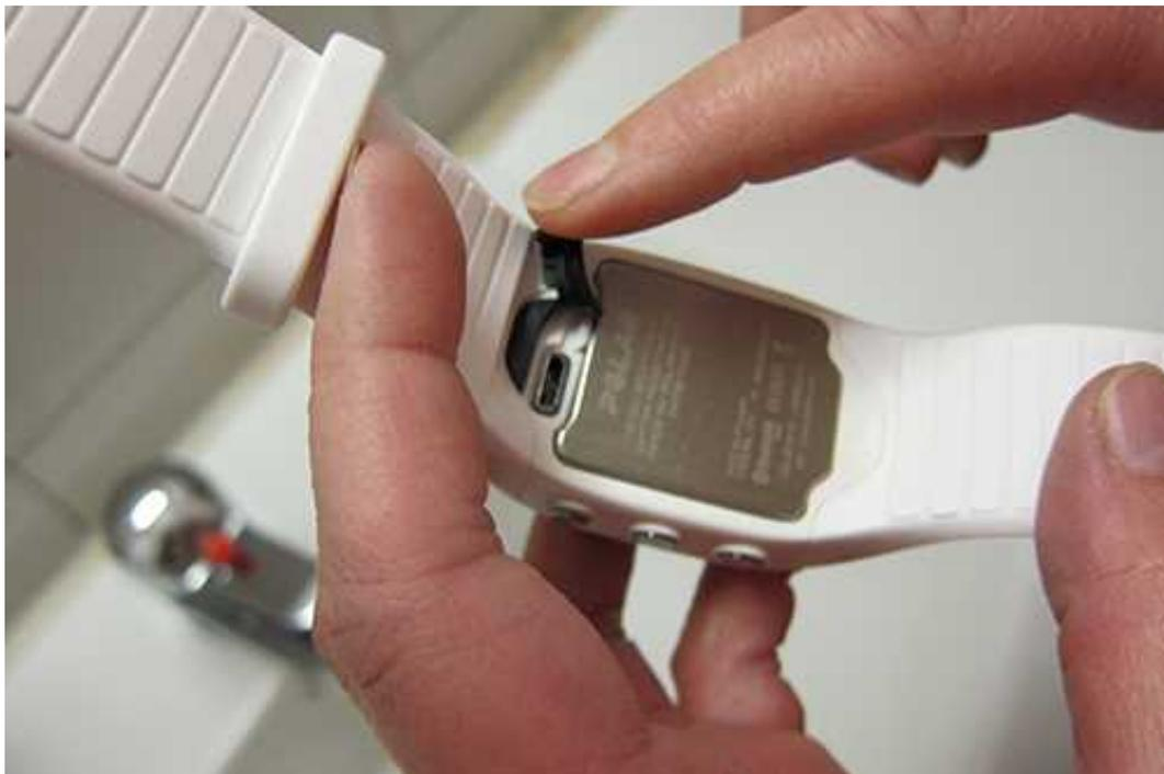
2. Rinse the USB port with lukewarm tap water. The USB port is water resistant and you can rinse it under running water without damaging the electronic components.
