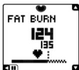
While in the desired zone, press OK for one second to lock. Fat burning zone locked or Fitness zone locked is displayed. The wrist unit gives a sound if you are training too hard or too light. For instance, fatburn zone is locked in this image. To unlock a zone, press OK for one second.
