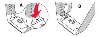
2. Plug the other end of the cable into your computer's USB port. Check that the USB port is dry before connecting it to the computer. If the battery is completely empty, it takes a couple of minutes for the charging to start.
