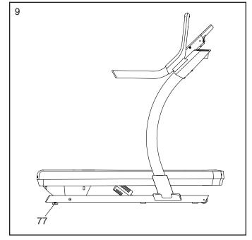
10. Make sure that all parts are properly tightened before you use the incline trainer. Keep the included hex keys in a secure place. One of the hex keys is used to adjust the walking belt (see page 25). To protect the floor or carpet from damage, place a mat under the incline trainer. To avoid damage to the console, keep the incline trainer out of direct sunlight.
