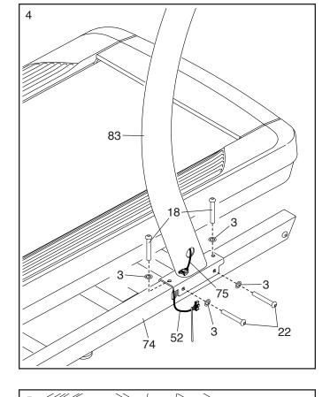
5. Connect the Base Wire (52) to the Upright Wire (75). IMPORTANT: The wire connectors should slide together easily and snap into place with an audible click. If they do not, turn one connector and try again. You must connect the wires properly for your incline trainer to function properly.
