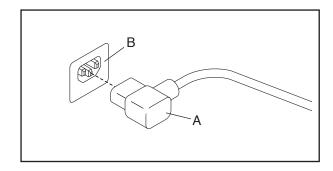
2. Plug the power cord into an appropriate outlet (C) that is properly installed and earthed in accordance with all local codes and ordinances.
