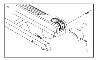
Next, locate the Reed Switch (113) and the Magnet (112) on the left side of the Pulley (42). Turn the Pulley until the Magnet is aligned with the Reed Switch. The gap between the Magnet and the Reed Switch must be about 1/8 in. (3 mm). If necessary, loosen the #8 x 3/4" Clip Screw (111), move the Reed Switch slightly, and then retighten the Clip Screw. Then, reattach the Left Foot Rail Cover (44), and run the incline trainer for a few minutes to check for a correct speed reading.
