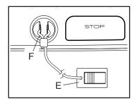
may take some time for the console to be ready for use. IMPORTANT: In an emergency, the key can be pulled from the console, causing the walking belt to slow to a stop. Test the clip by carefully taking a few steps backward; if the key is not pulled from the console, adjust the position of the clip.
