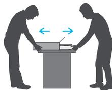
2. Unpacking and setting up the DT2 is a two person job. Once removed from the packaging, have a colleague assist you to place the DT2 on your existing work surface.
