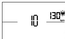
During the **Training Session and active pulse measurement**, press the Recovery Pulse key. After 10 seconds the measurement will begin.
