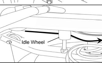
2.Next, thread the Belt around the Idle Wheel as shown. Once around the Idle Wheel, attach the Rower Belt to the Belt/Bungee Pulley. There is an obvious "lip" at the attachment point.
