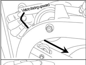
Begin reattaching the Rower Belt by threading around the Rower Belt Pulley with the Velcro side facing upward as illustrated.
