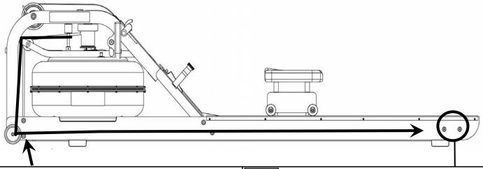
Hint: Before reattaching the Inner Clip/ Bungee Hook End Frame, tie a slip knot under slight tension at the lower bungee pulley. This will keep the bungee under tension while reassembling the Bungee Hook End Frame.
