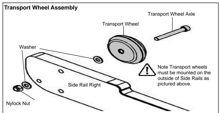
Once the Rear Brace and Side Rails are assembled, mount the Transport Wheel Assembly onto the Left/Right Side Rails.
