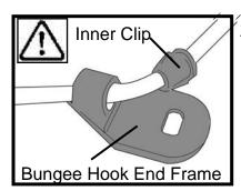
2.Unhook the Bungee Shock Cord from the Rear Leg. Then, push out the Inner Clip from the Bungee Hook End Frame. Pull the Bungee through the Inner Clip until free. This will allow for the Bungee Shock Cord to be threaded completely out of the Main Frame and up to the Belt Bungee Pulley where it will be re-attached once the Rower Belt is in the proper position.
