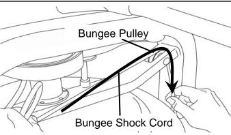
4.Rethread the Bungee Shock Cord (on opposite side of the Idle Wheel) back through the Bungee Pulleys and tie off at the Attachment Point.
