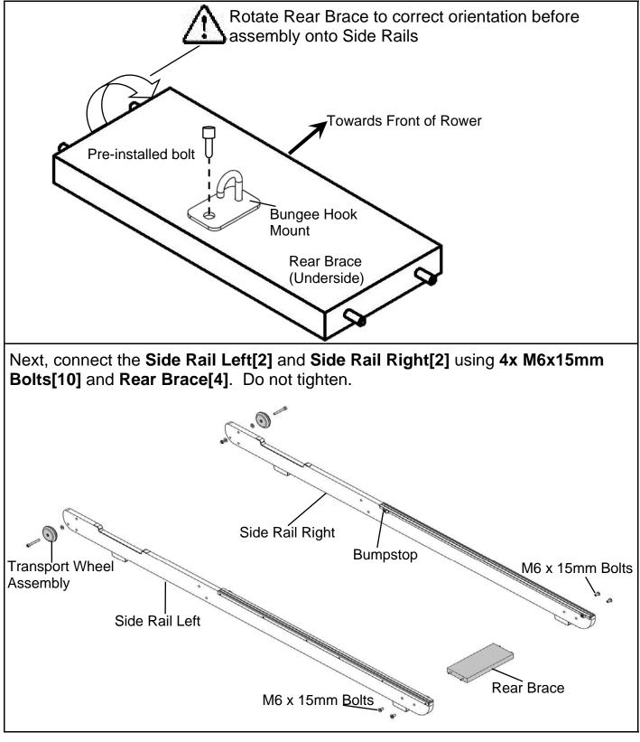
Tip: Bumpstops facing inside of rail for correct assembly orientation.
