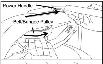
3. Wind the Rower Belt onto the Belt/ Bungee Pulley until the Rower Handle is as it's furthest forward position.
