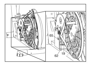
When the Drive Belt (19) is tight, tighten the M8 x 22mm Screw (65).
