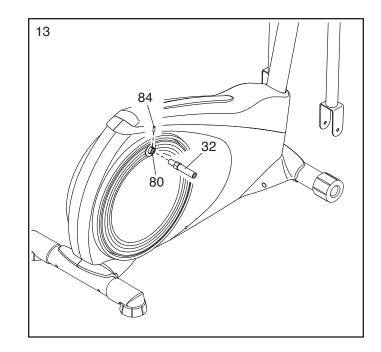
14. Apply a small amount of grease to the axle on the right Crank Arm Stud (32).
