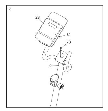
8. Insert the excess wire into the Upright (2).
