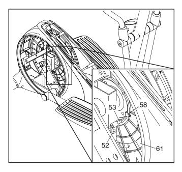
Next, rotate the Pulley (61) until a Magnet (58) is aligned with the Reed Switch (53). Slide the Reed Switch slightly toward or away from the Magnet. Then, retighten the M4 x 16mm Screw (52). Plug in the power adapter and rotate the Pulley for a moment.
