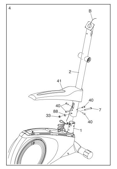
See the inset drawing. Locate the wire tie (B) in the lower end of the Upright (2). Tie the wire tie to the Main Wire (73). Next, pull the upper end of the wire tie until the Main Wire is routed through the Upright.
