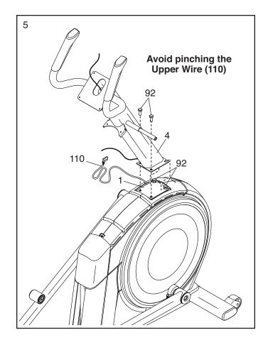
Locate the wire tie (A) in the lower end of the Upright (4). Tie the wire tie to the Upper Wire (110). Then, pull the upper end of the wire tie until the Upper Wire is routed through the Upright.
