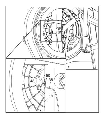
Next, slightly loosen the two indicated #8 x 1/2" Screws (50). Slide the Reed Switch (38) slightly closer to or away from the Magnet (43), and then retighten the Screws.
