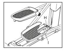
To lower the ramp, press the latch button (H), pull the ramp handle (I), and lower the ramp to the desired incline level. Then, release the latch button and engage the latch pin into one of the adjustment holes in the frame. Make sure that the latch pin is firmly engaged in one of the adjustment holes in the frame.
