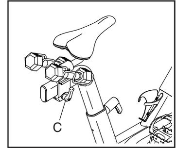
Note: The carriage handle (C) functions like a ratchet. Turn the carriage handle in the desired direction, pull it outward, turn it in the opposite direction, push it inward, and then turn it in the desired direction again. Repeat this process as many times as necessary.
