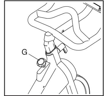
**IMPORTANT:** When the exercise bike is not in use, tighten the brake knob (G) completely.
