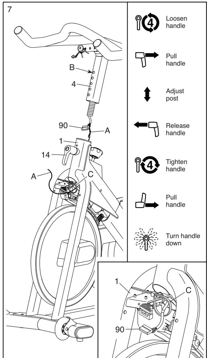
8. **See the inset drawing.** Connect the Upper Wire (90) to the Lower Wire (82). **Tip: The wire connectors should slide together easily and snap into place with an audible click. If they do not, turn one connector and try again.**
