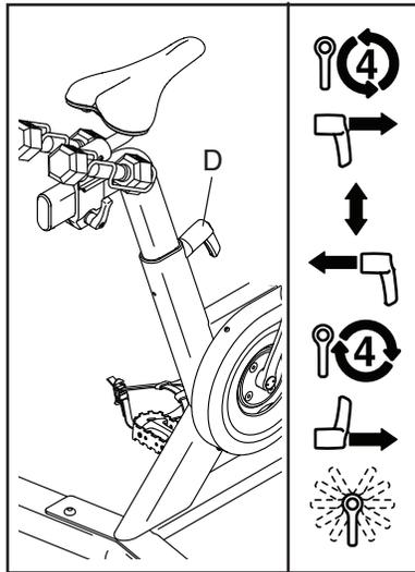
**Make sure that the adjustment handle is engaged in an adjustment hole.** Then, pull the adjustment handle outward, turn it so that it points downward as shown, and then release it.
